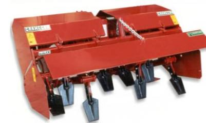
**UK** Changing the tools of the decompactor, it can be converted to operate as a spading machine with a soil-engaging depth of 30 cm.
