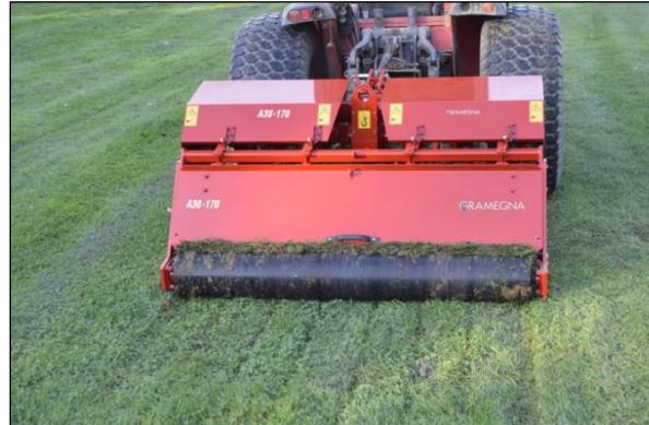
**UK** The machine is equipped with steel knives of curved profile capable of penetrating the soil to a depth of 20-22 cm.
